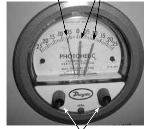
Pressure Setting Knobs Photohelic® Gauge
