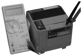
DC Voltmeter and Flame Amplifier
