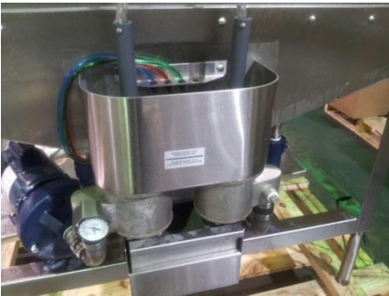
5AGES sump, drain ball, water-level decal, chemical tubes, scrap box
