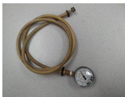
Spray arm pressure tester #088-1048
