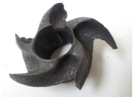
Impeller damaged from high acid solution
