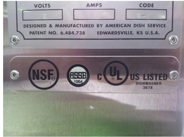
Typical name plate information and listing marks
