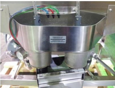
Showing sumps, drain balls, water-level decal, chemical tubes
