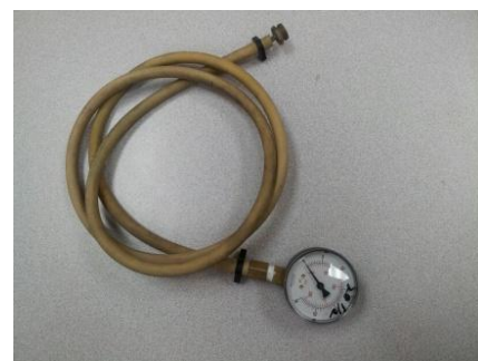
Spray arm pressure tester #088-1048
