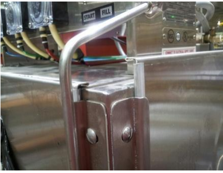
Showing ❌ misaligned arms on corner
