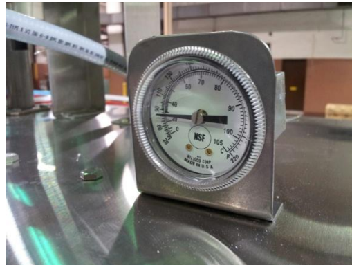
Tank temperature indicator located top of hood
