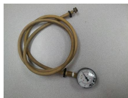
Spray arm pressure tester #088-1048
