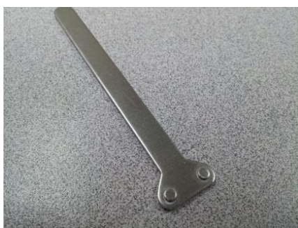
Cam adjusting tool
