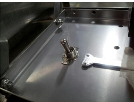
De-lime switch in control box
