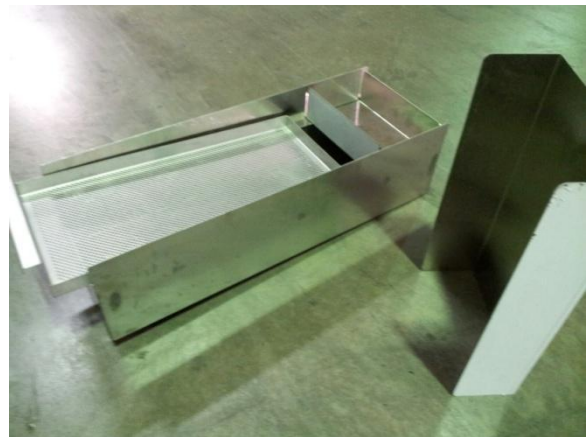
5-CD scrap box assembly, tray, spacer, cover
