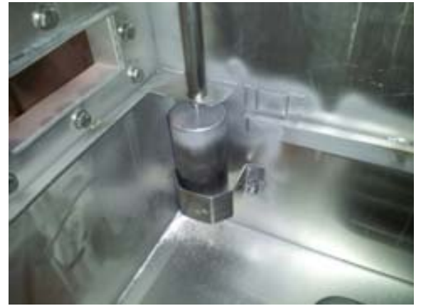
Wash tank float and tank overflow
