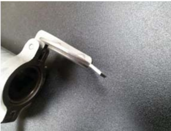
Tab on endcap bent inward, causing loose fit
