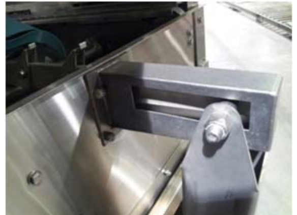
Rocker arm attached to conveyor bar, drip chute
