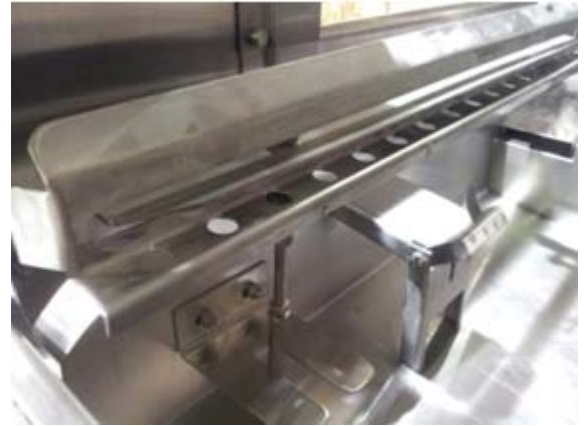
Wash tank sequence bar, pendulum with magnet
