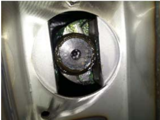
Cam bearing screws into cam block B
