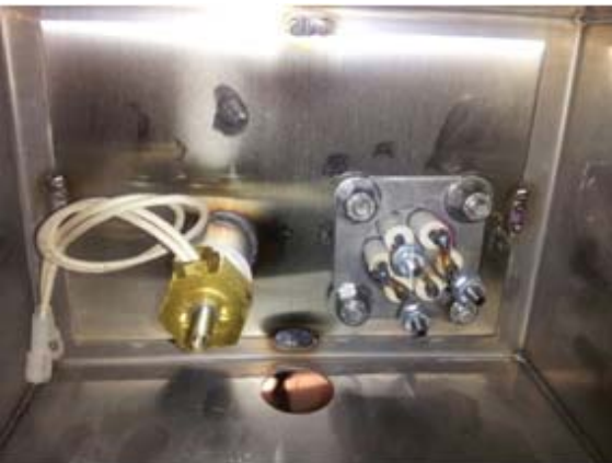
Wash tank thermostat, rotate center rod Left to increase
