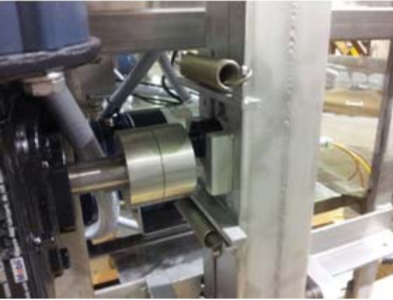
Conveyor drive, cam blocks, bearing, clutch springs (use caution)
