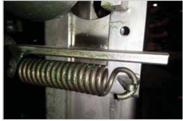
Rocker arm slip clutch spring, hook to bar weldment
