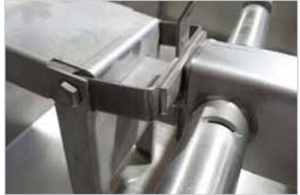
Arm resting in "T" index with latch down
