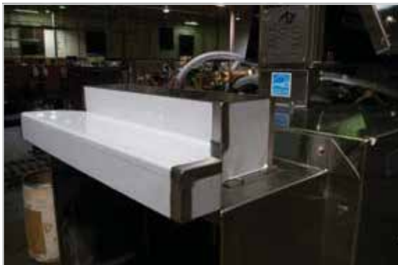
Vent attachments to end shield, 4" x 16" opening
