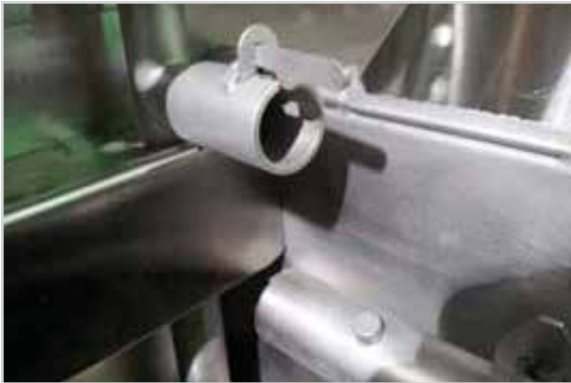
Showing pumped rinse manifold locking tab
