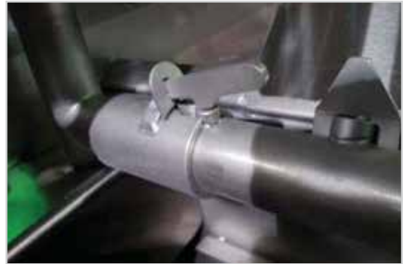
Rinse arm index notch, latch will drop as arm is pushed in
