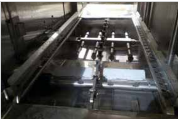
Travel through conveyor tray rails, center pull bar w/dogs
