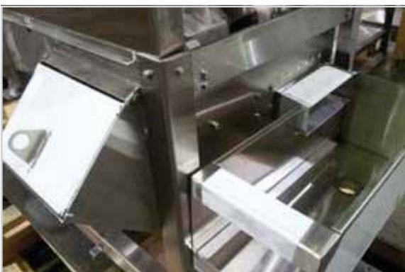
ADC-66 power scrapper, overflow to scrap box
