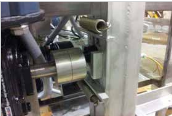
Conveyor drive, cam blocks, bearing, clutch springs (use caution)
