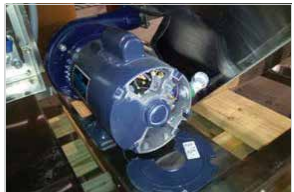
66 power scrapper motor, 1.5 HP, 208v, single-phase
