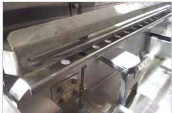
Wash tank sequence bar, pendulum with magnet
