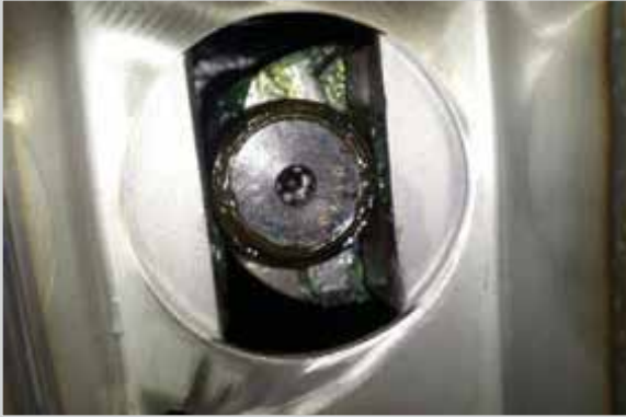
Cam bearing screws into cam block B
