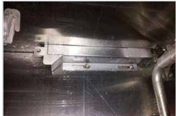
Showing diverter slide to fill both tanks
