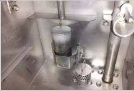
Rinse tank float, pump filter, pumped rinse manifold
