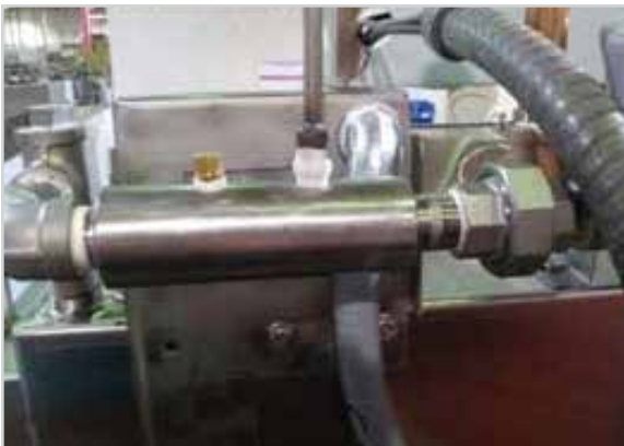
Mixing chamber with two 1/8" pipe threaded ports Hi-temp mixing chamber is SS, Chemical is a polymer
