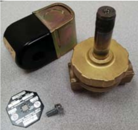
Remove screw and coil from tube
