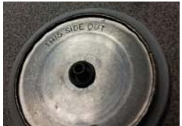
Installing diaphragm upside down, see lettering up
