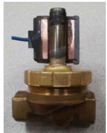
Coil will lift plunger in the tube.
