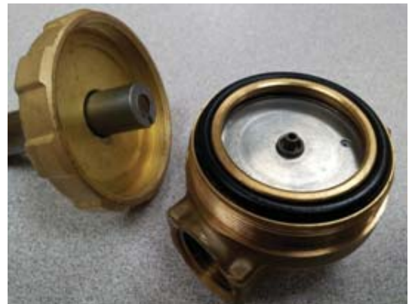
Twist to remove top, RH threads, first close water pressure to valve then twist top
