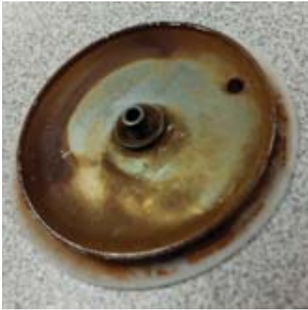
Errors are returning a corroded diaphragm to service.
