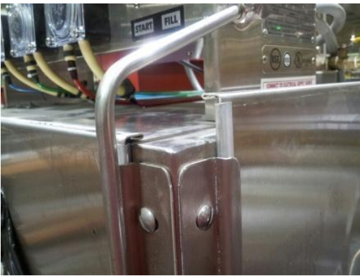
Showing misaligned arms
