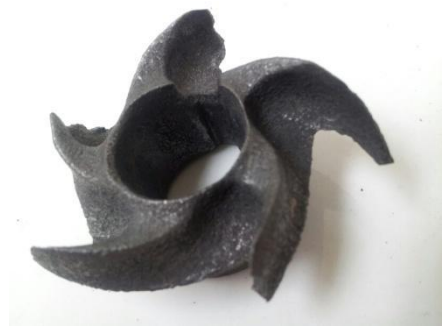
Impeller damaged from high acid solution
