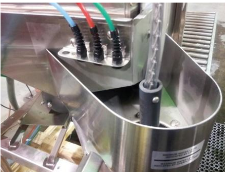
Showing sump, drain ball, water-level decal, chemical tubes
