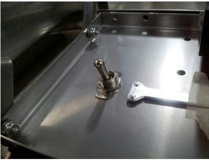
De-lime switch in control box
