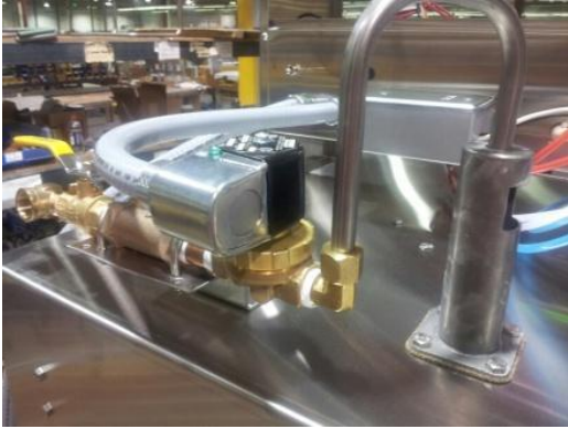
Showing ½” female pipe inlet, ball valve, y-line filter, water solenoid, ASSE approved air gap (backflow preventer)
