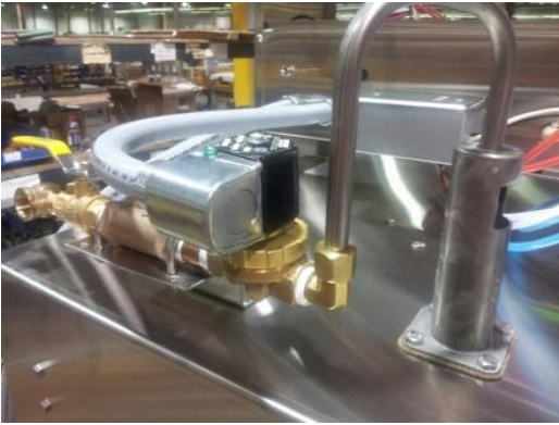
Showing ½” female pipe inlet, ball valve, y-line filter, water solenoid, ASSE approved air gap (backflow preventer)
