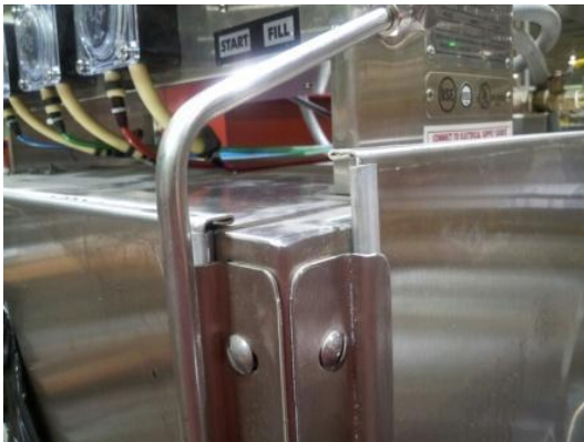
Showing misaligned arms
