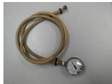
Spray arm pressure tester #088-1048
