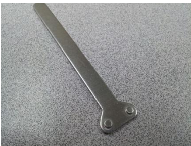
Cam timer adjusting tool
