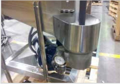
Showing AF-ES sump, drain ball, thermometer
