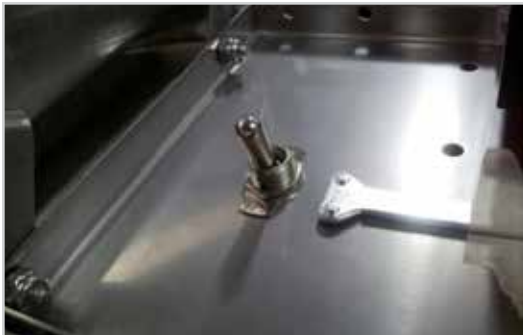
De-lime switch in control box
