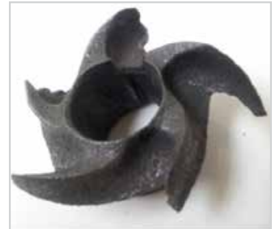
Impeller damaged from high acid solution
