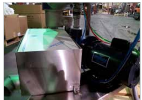
Rear view of installed side exit ES scrap box
