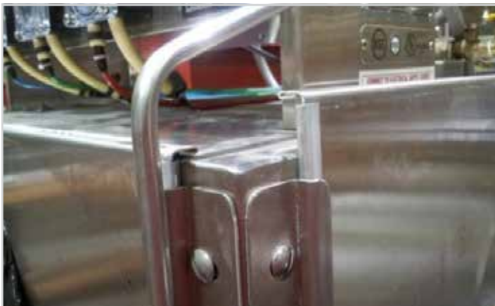
Showing misaligned arms
