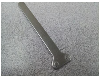
Cam timer adjustment tool #088-1048
