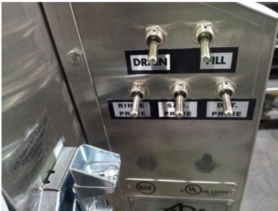
Showing controls on lower access door
