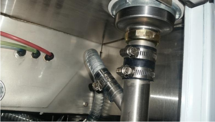
Drain hose connection to drain pipe
