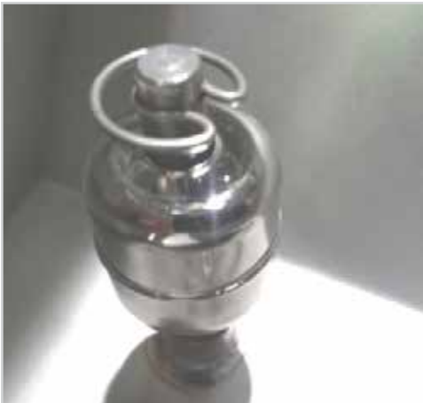
Control float, "O" mark should be on top
