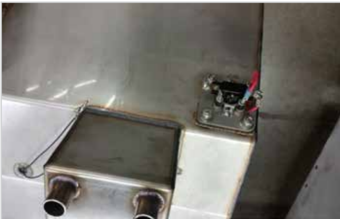
Showing bottom of tank, float wire, sump, heater attached
