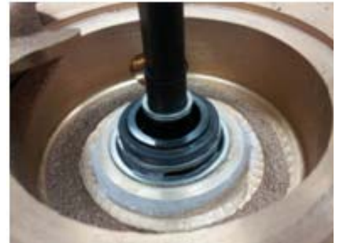
Graphite seal pressed into pump base
