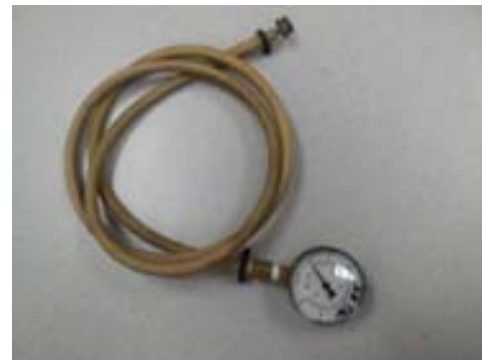
Spray arm pressure tester #088-1048
