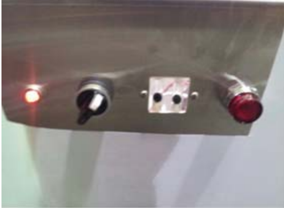
Cycle light, master switch, chemical sight window, start switch
