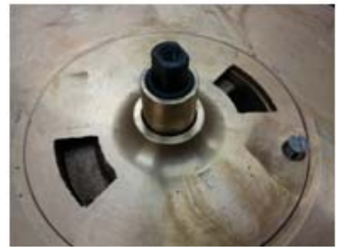
Drain inlet plate, w/alignment screw
