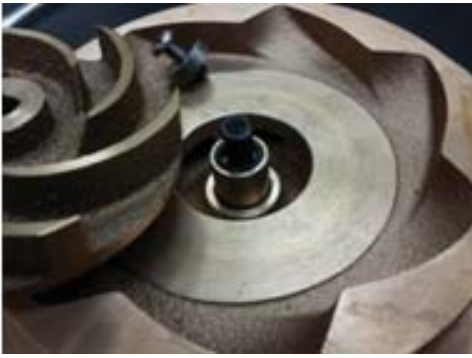
Impeller removed from housing
