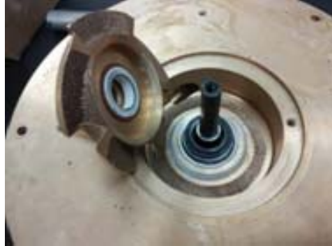
Ceramic seal pressed into propeller
