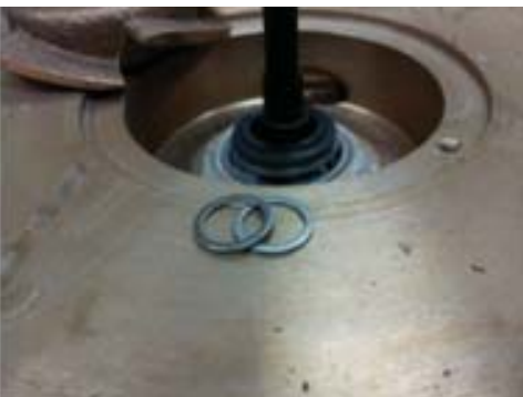
2 Spacer washers under propeller
