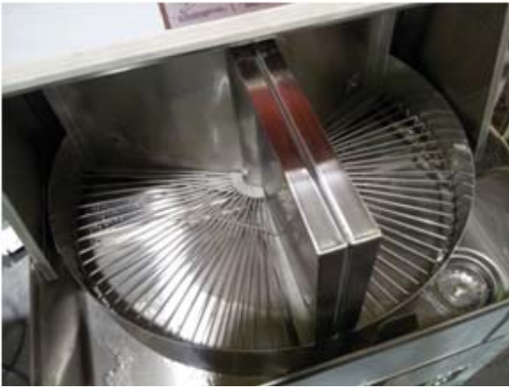
Carousel is rotated manually, shows correct position for cycle
