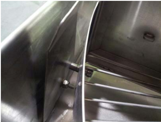
Latch located between the carousel and the glasswather cabinet.
