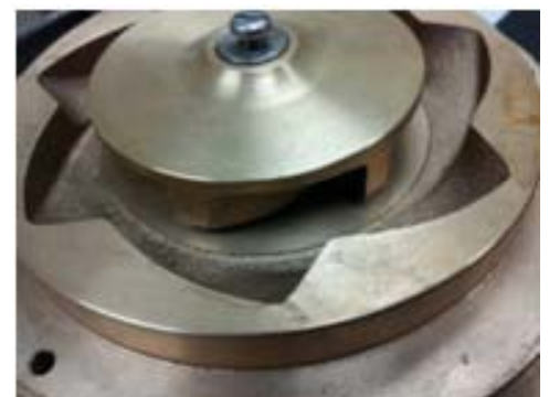
Diffuser removed, centrifugal Impeller
