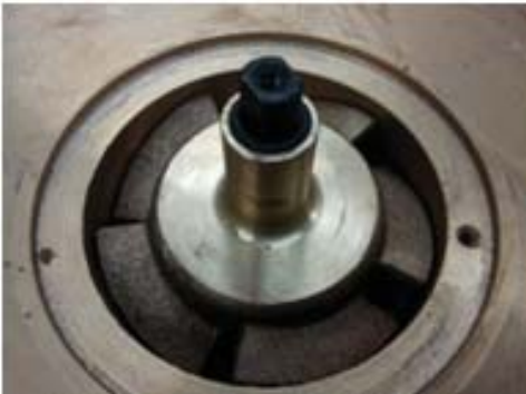
Drain axial propeller, o-ring on shaft
