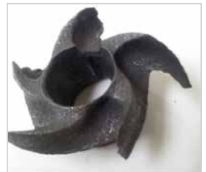
Impeller damaged from high acid solution
