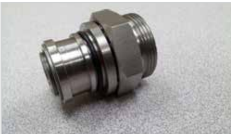
Spray arm bearing with sealing o-ring
