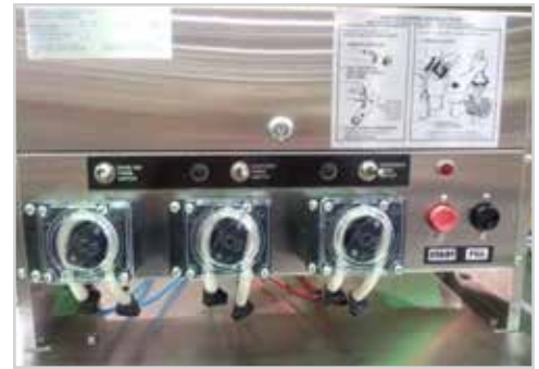
Showing detergent, rinse, sanitizer external pumps
