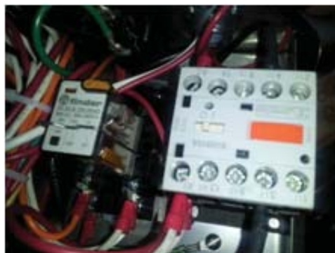
Left is Start Relay, right is Heater Relay Left is Drain Relay, right is Heater Contactor Optional buzzer for low chem. alarm
