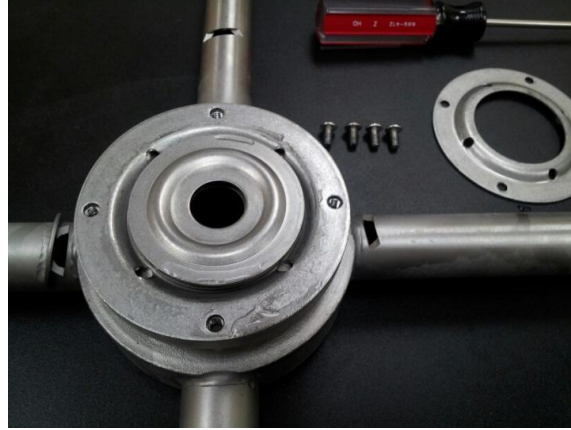
Remove top shell, exposing top bearing race
