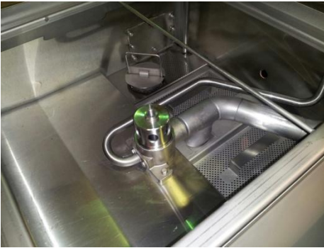
Showing spray arm base & transfer tube
