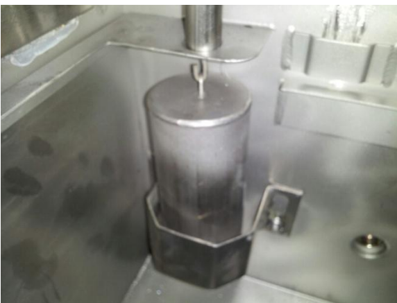
Wash tank float and tank overflow
