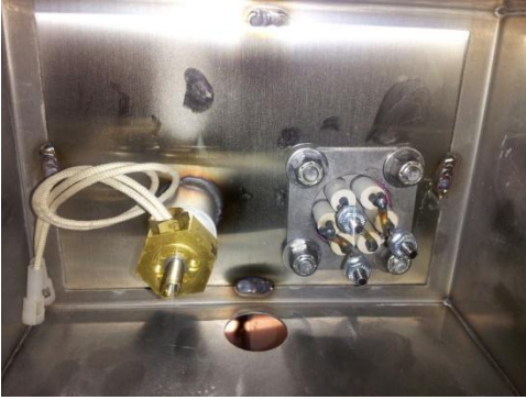
Showing thermostat and sustainer heater terminals*
