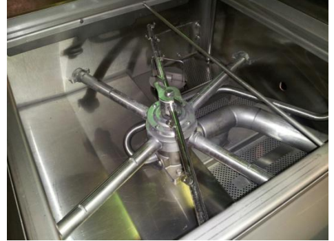
Final rinse arm twisted into transfer tube
