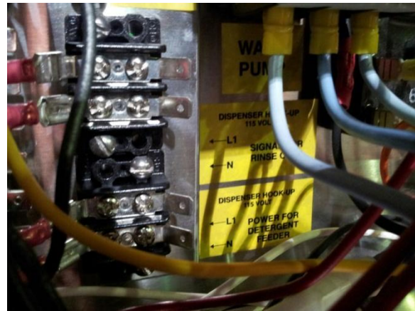
Showing dispenser signal connection terminals
