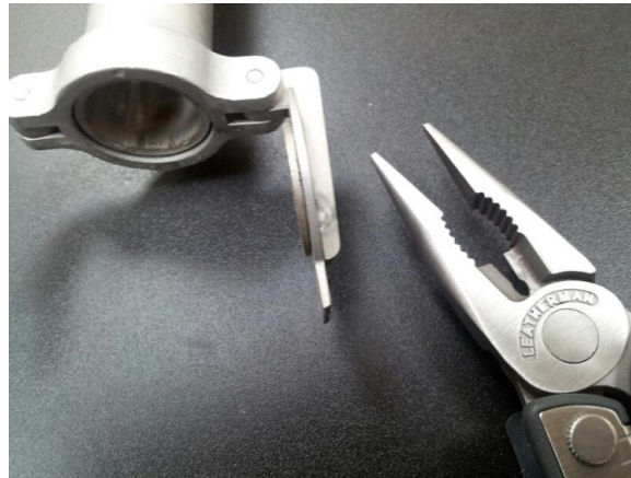
Straighten tab in line with the coin edge to tighten
