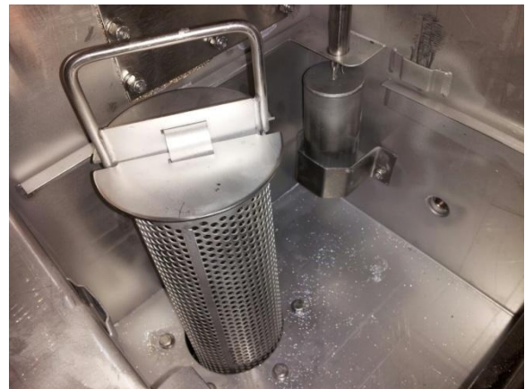
Pump filter in drain sump
