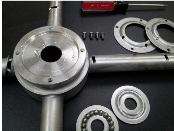
Races are interchangeable, capture shells are also
