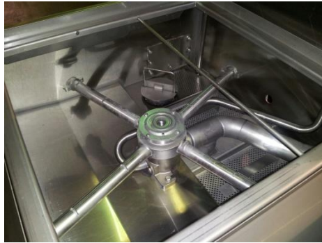
Wash arm w/bearing installed on base
