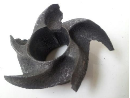
Impeller damaged from high acid solution
