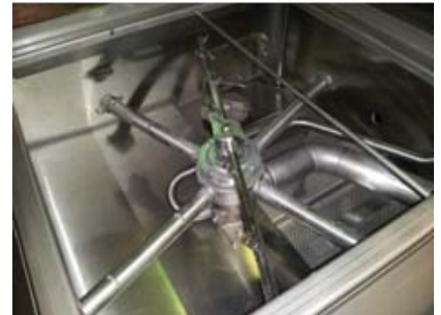
Final rinse arm twisted into transfer tube
