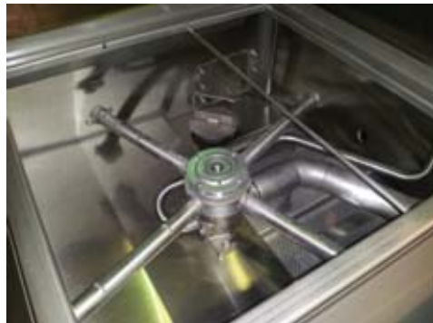
Wash arm w/bearing installed on base
