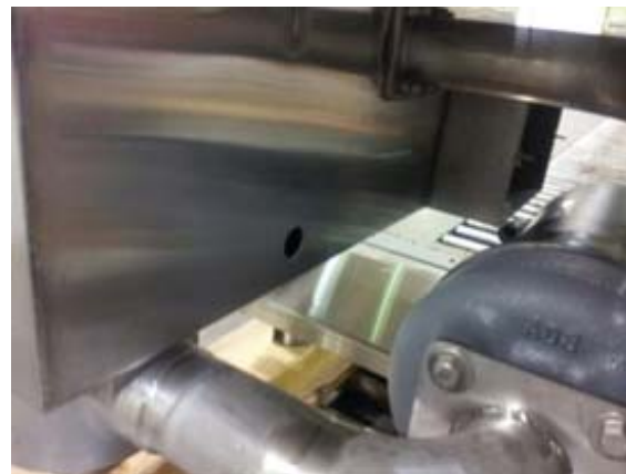
Showing 7/8" detergent probe hole behind pump motor
