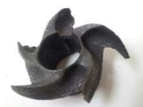
Impeller damaged from high acid solution
