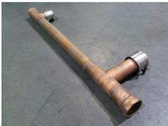
HT-25 drain manifold with "no-hub" connectors
