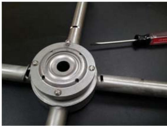
Remove 4 screws and lift top shell
