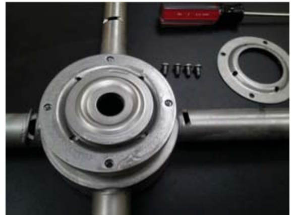
Remove top shell, exposing top bearing race
