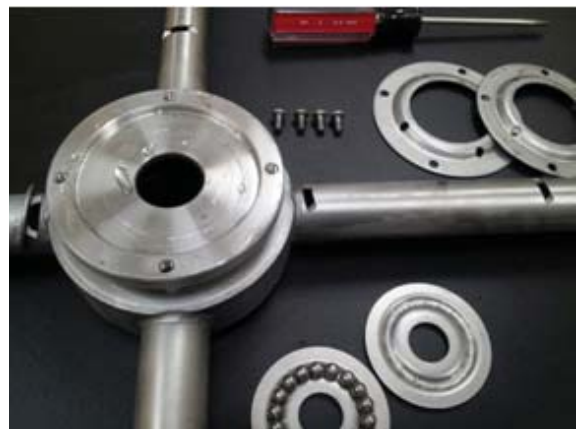
Races are interchangeable, capture shells are also
