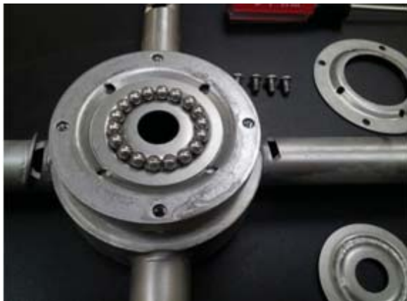
Top race removed, ball bearings for replacement
