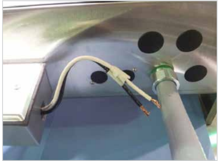
Showing power connection box for 120v wiring
