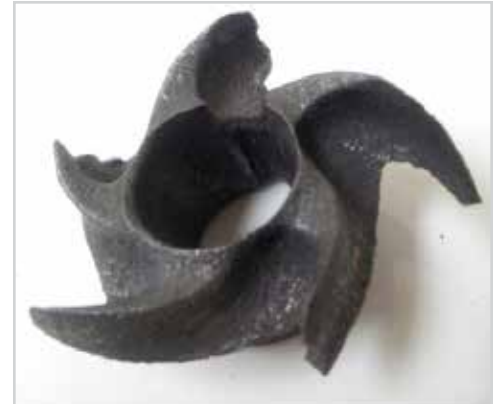
Impeller damaged from high acid solution
