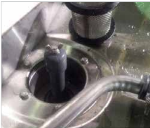
Showing sump, drain ball, pump filter
