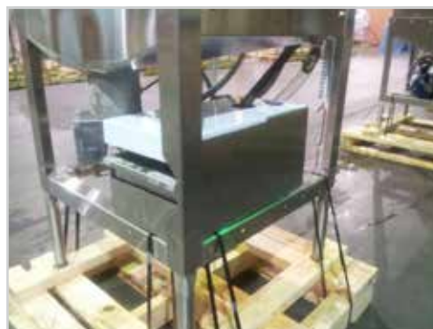
L-3DW-S scrap box in-frame mounting
