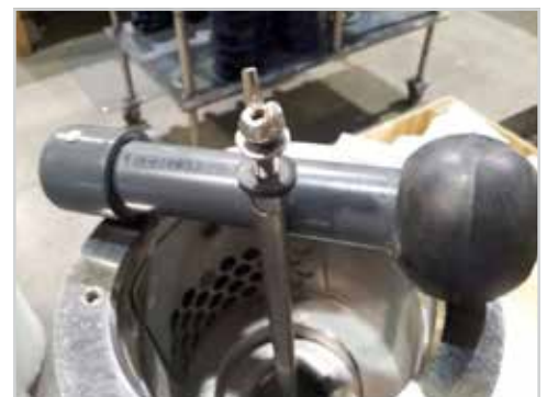
Drain ball assembly, note rubber washer on push rod
