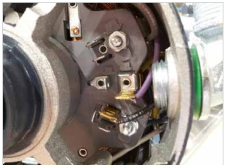
Line connection spades for L1, Neu (arrow 1 & 2)
