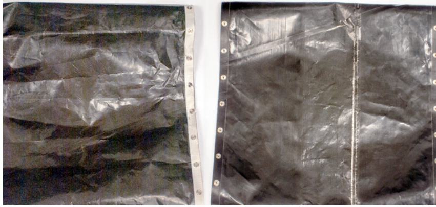
Examples of damaged belts
