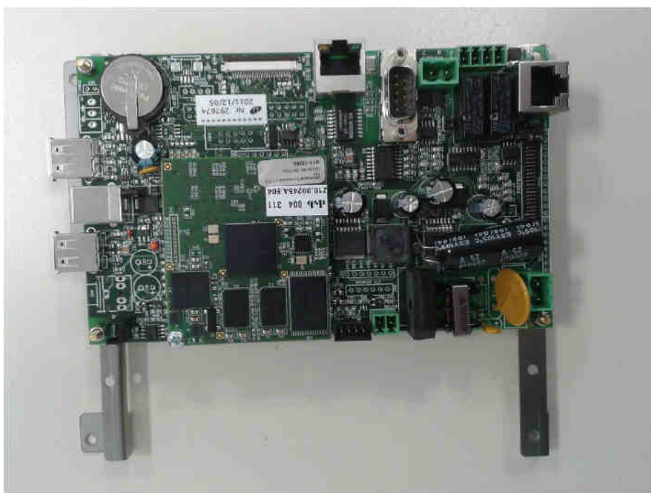
CPU board mounted with KIT
