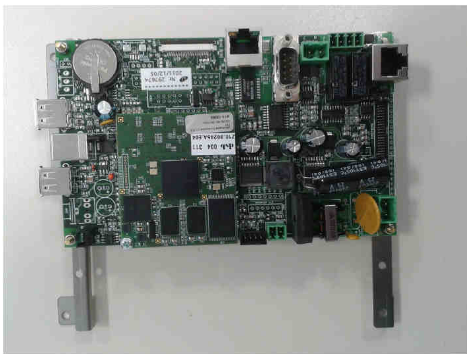
CPU board mounted with KIT
