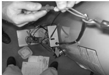
Checking continuity of upper sensor wire harness.
