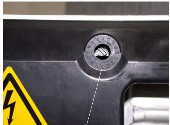
Switch cover 360-480 with setting scale for encoded switch
