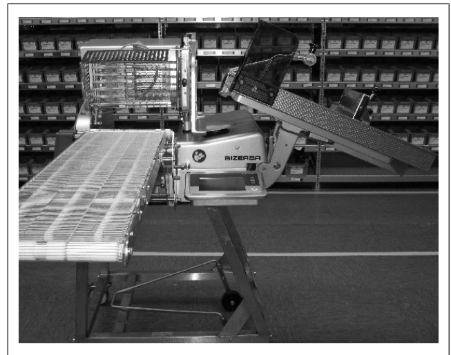
Fig. 97: Tilting the carriage outwards
