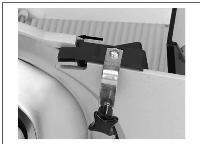
Fig. 148: Clamping the sharpener
