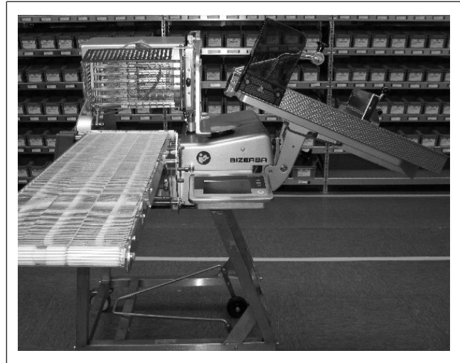
Fig. 87: Tilt the carriage to the outside
