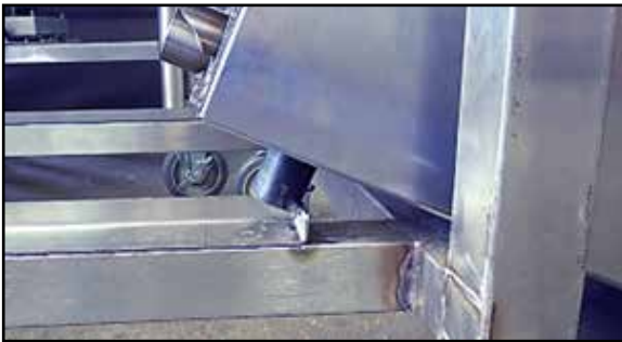
Rear feet being lifted over front welded stops
