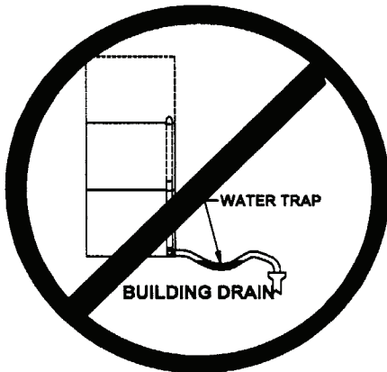
IMPROPER DRAIN LINE CONNECTION
