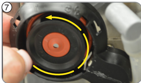
7. Rotate tab on mixing chamber bases further counter clockwise, and remove from shafts by pulling straight out.
