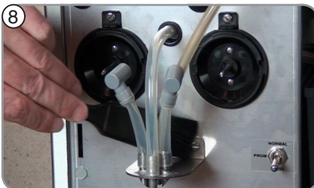
8. Use flat brush to clean dispense tube connectors area.
