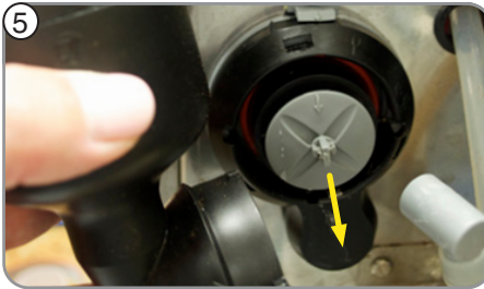
5. Remove mixing chambers by pulling straight out.
