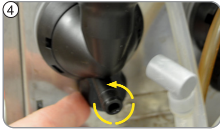
4. Rotate tab at bottom of mixing chamber bases. Twist counter clockwise to release bases.
