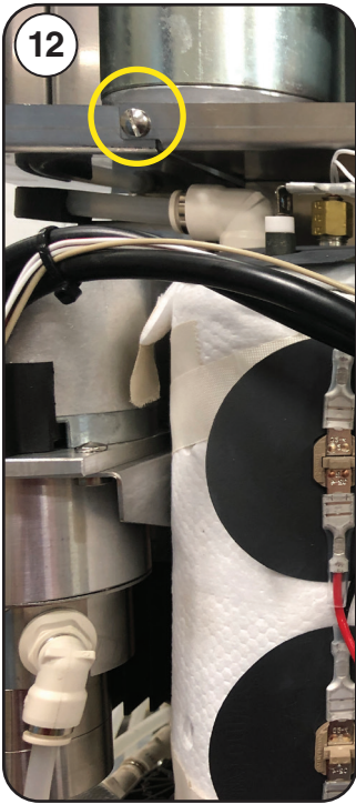
Remove the 2 slotted screws above the tank module.
