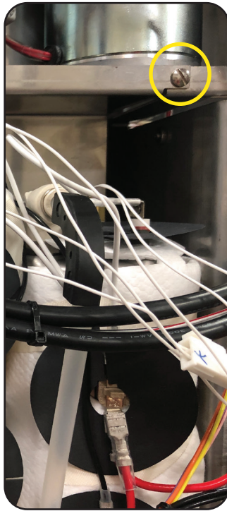
Remove the 2 slotted screws above the tank module.
