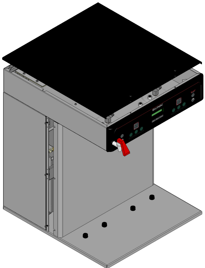
FIG. 10-3 ICB/ITCB HV TWIN COMPONENT ACCESS
