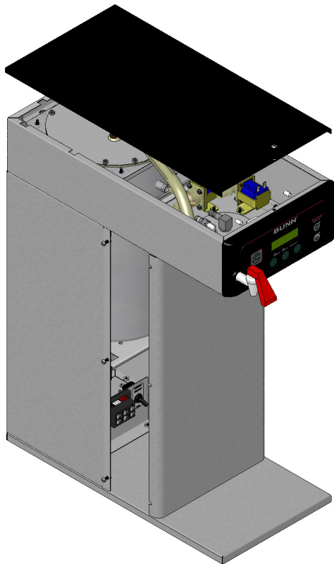
FIG. 10-1 ICB/ITCB HV COMPONENT ACCESS
