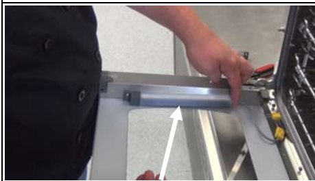
Fig. P 11) Slide the light cover into the top bracket, making sure the white side of the cover is facing up.
