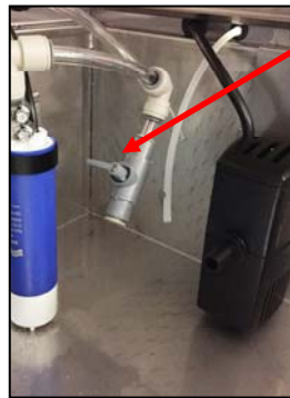
Fig. 3 Priming valve in OPEN position
