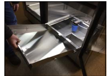
Fig. 1 Access the water reservoir; the sensor will be on the left side
