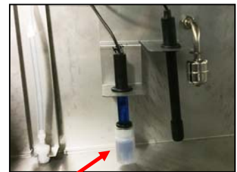
Fig. 2 Blue PH sensor (shown with cap on)
