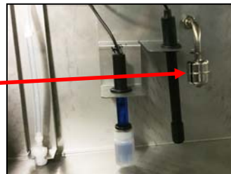
Fig. 2 Float switch/sensor; left side of reservoir; shuts off water once filled to proper level
