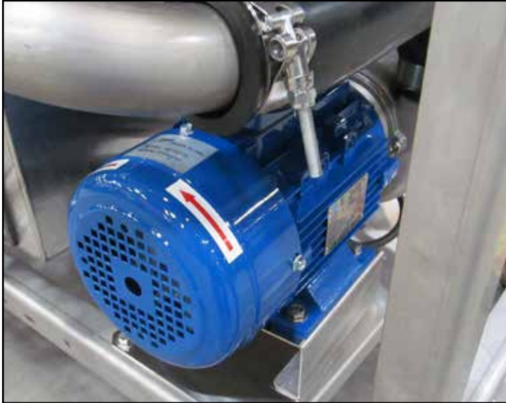
Fig. 23 - Motors rotate counter-clockwise.
