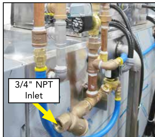
Fig. 5 - No booster may not require a PRV.
