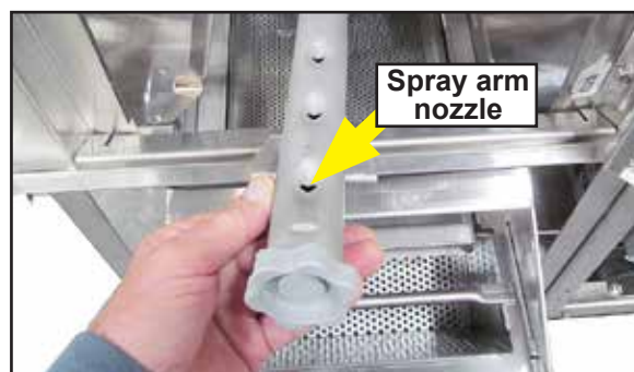
Fig. 68 - Make sure spray arm nozzles are clear.
