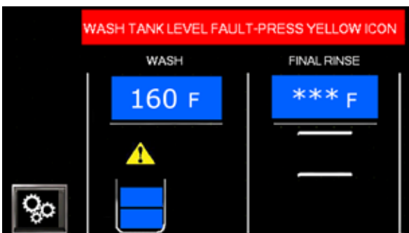
Fig. 25 -Wash Tank Level Fault
