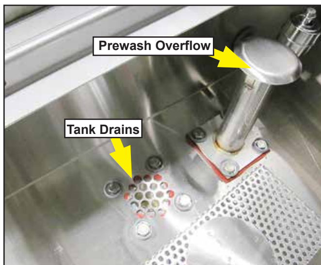
Fig. 72 - Tank drain prewash overflow
