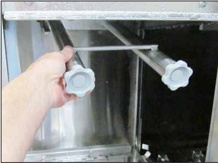
Fig. 80- Slide spray arm on tracks toward standpipe manifold.
