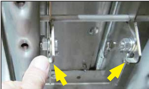
Fig. 64 - Press latches to release upper spray arm.
