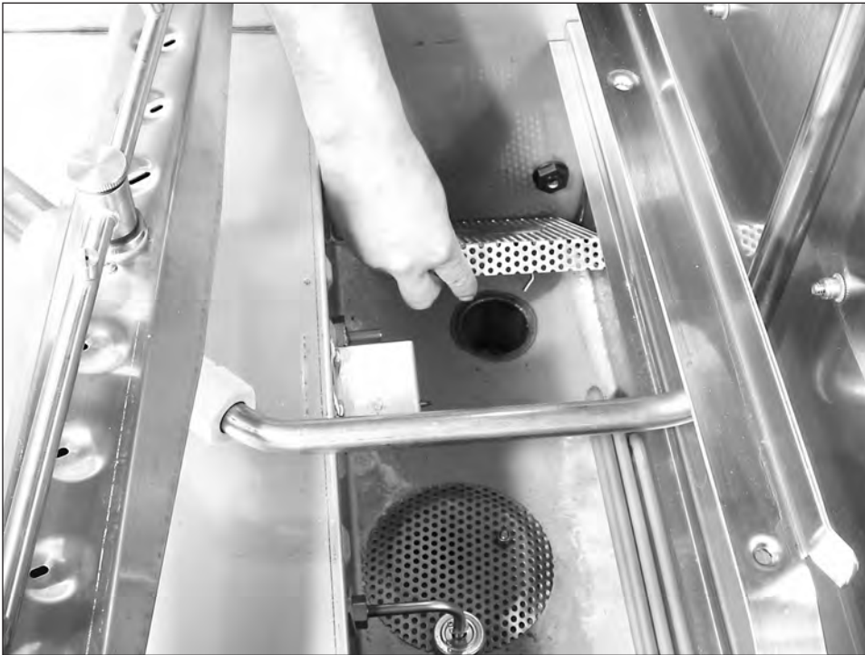
Make sure tank is clean, the pump intake screen is installed and the float switch moves freely.
