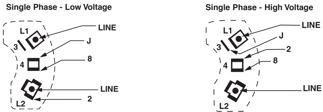
Figure 17 Pump Motor Wiring Diagrams
