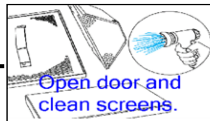
Fig. 85 - Clean scrap screens
