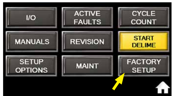
Fig. 61 - Factory Setup not available for supervisors.
