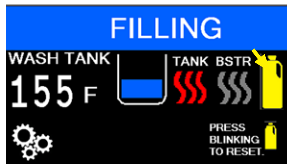
Fig. 37 - LOW DETERGENT ALERT - (flashing bottle)
