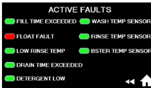
Fig. 56 - ACTIVE FAULTS screen
