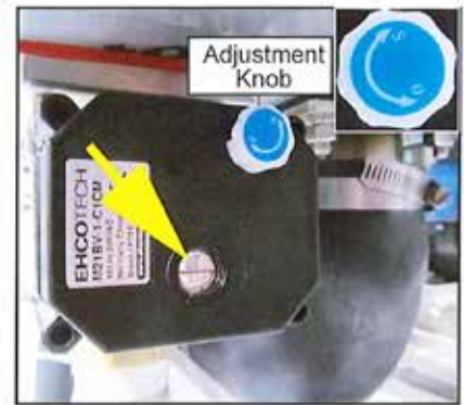
Type 2 - With adjusting knob
