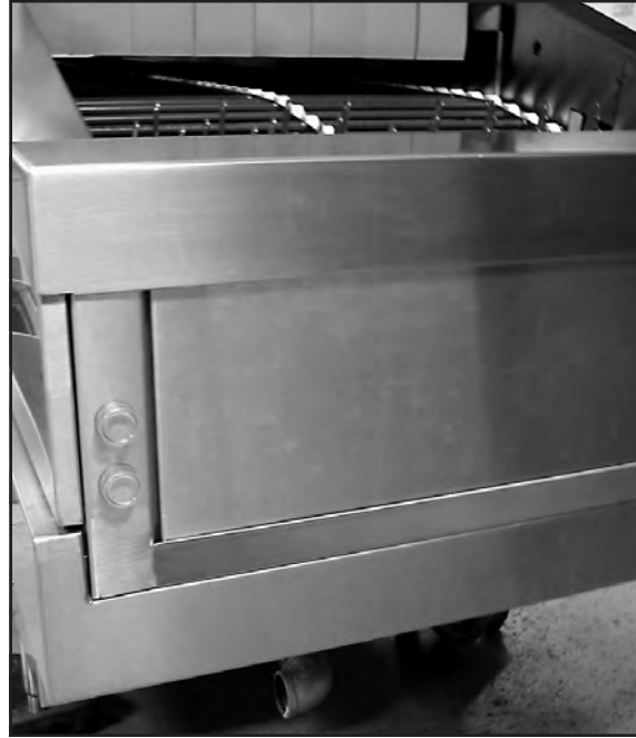
Load-end Start-Stop Station
