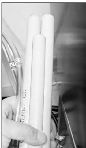
Chemical Pick-up Tubes, stiffener tubes & line strainers.
