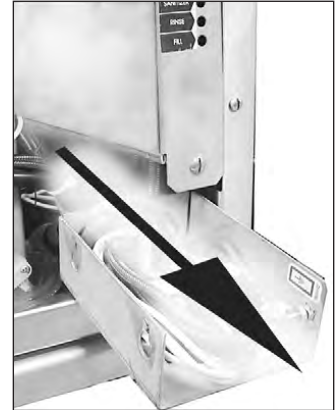
Pull the MTB out to wire main incoming power.
