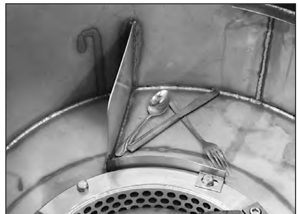
A powerful magnet is in the pulper grinding chamber. The magnet will attract utensils and other metal objects if they contain enough iron in their composition.
