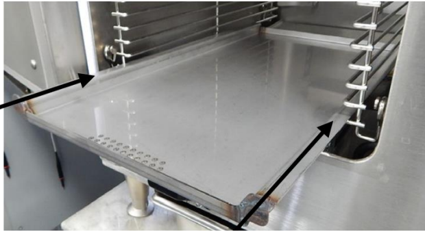
Figure 3-9 Bypass Shield Installation
