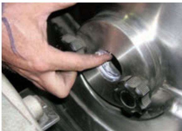
7. Grease seal with food grade grease.
