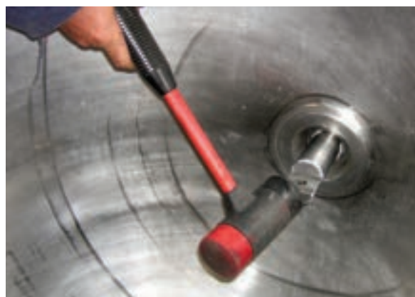
10. Tap shaft back to seat up against retaining ring.
