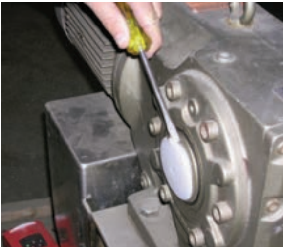
2. Remove shaft end cap.
