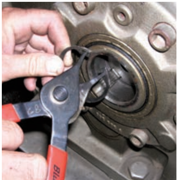
4. Remove shaft retaining ring.
