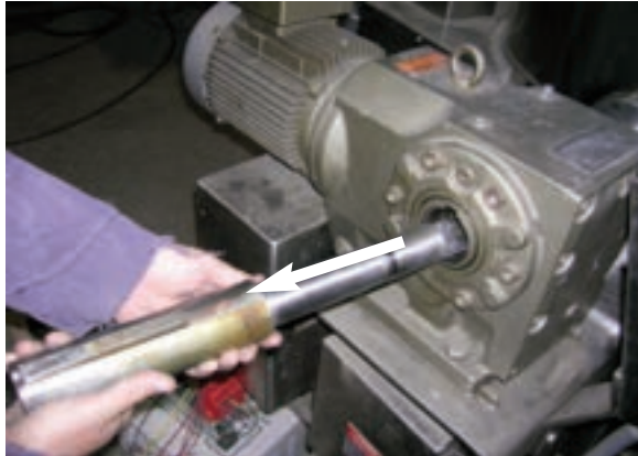
5. Gently hammer out shaft and remove.
