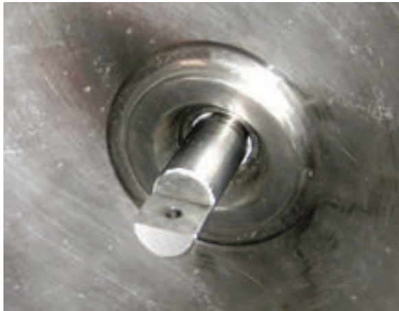
1. Remove mixer arm leaving flat surface on drive shaft facing upwards.
