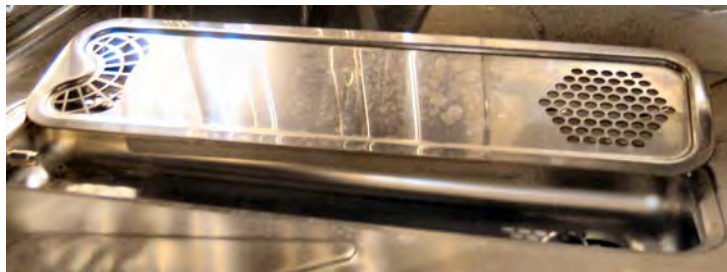
Drain Cover and Drain
