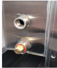
Sanitizer line before and plugged
