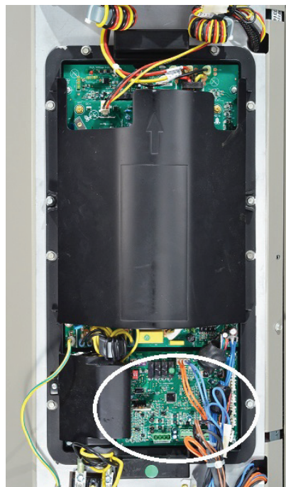
Fig. 26 - AOC (Application Operational Control) Board
