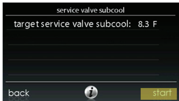
Fig. 16 - Service Valve Subcool Target Value
