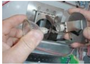
Fig. 4.4 Substitute light bulb.
