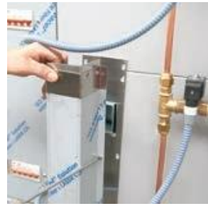
Fig. 6.1 Loosen the back steam output.
