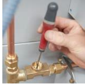
Fig. 7.5 Check if the piston is damaged or dirty, clean or substitute it. Reassemble the solenoid and open the water valve.
