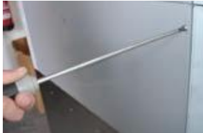
Fig. 2.1 Loosen the screws on the left side panel.
