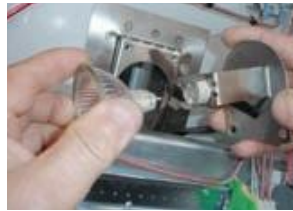
Fig. 4.4 Substitute light bulb.
