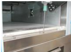
Fig. 5.1 Loosen lower frame screws.
